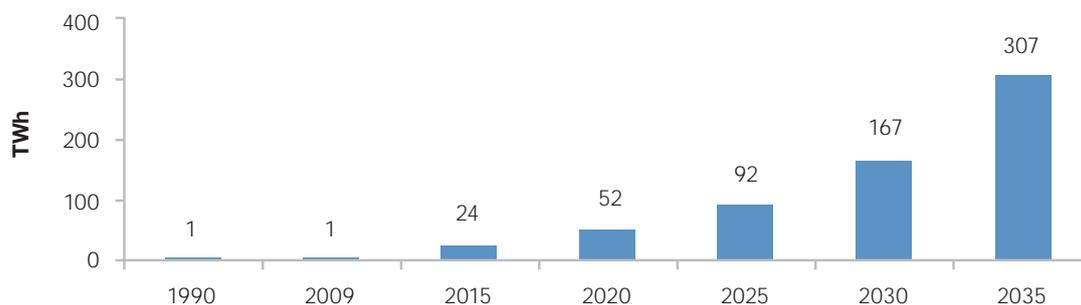
**Figure 2-16 | Global CSP energy generation to 2035 [weo11]**
