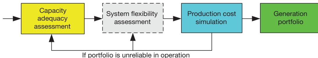
Figure 4-5 | Generation planning process incorporating flexibility assessment [trp11]
