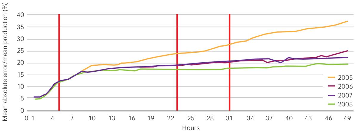
**Figure 3-21 | Wind forecast error as a percentage of wind production, as a function of the time forward from the present [uei10]**
