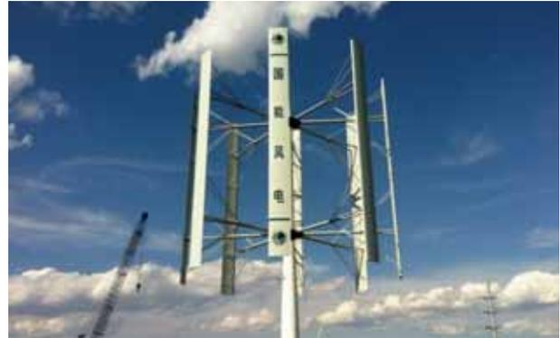
**Figure 3-4 | Vertical-axis turbine** (Xu Ji)
