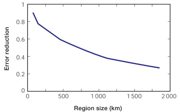
**Figure 3-20 | Decrease of wind forecast error for aggregated wind power production [hol09] (energy & meteo systems)**
