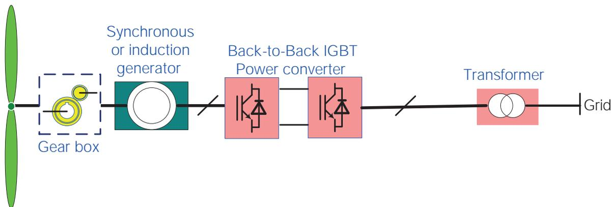
**Figure 3-9 | Topology of a full-power conversion WTG (SGCC)**
