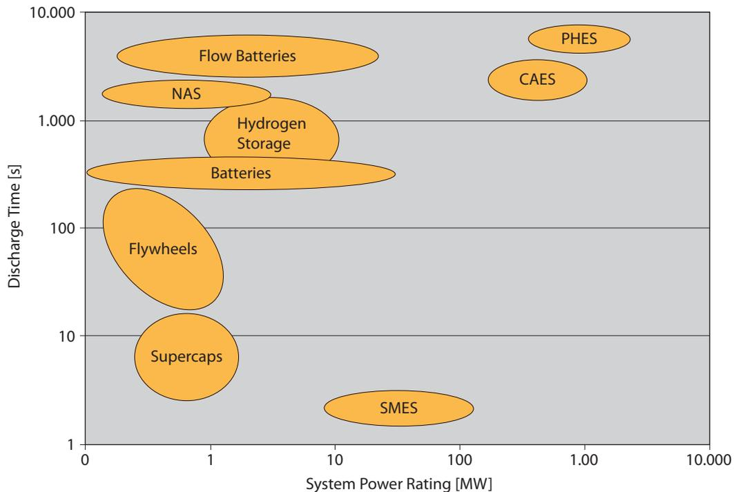
Figure 1. Comparison of different storage systems
