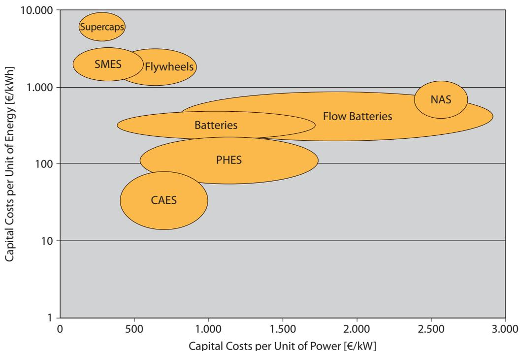
Figure 3. Rough comparison between current costs of storage systems
