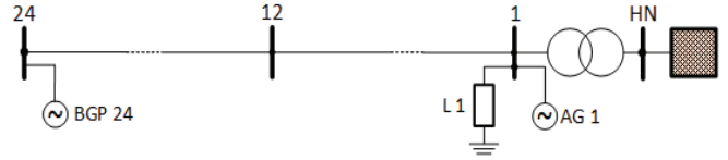
Fig. 3: Scheme of the radial test system
