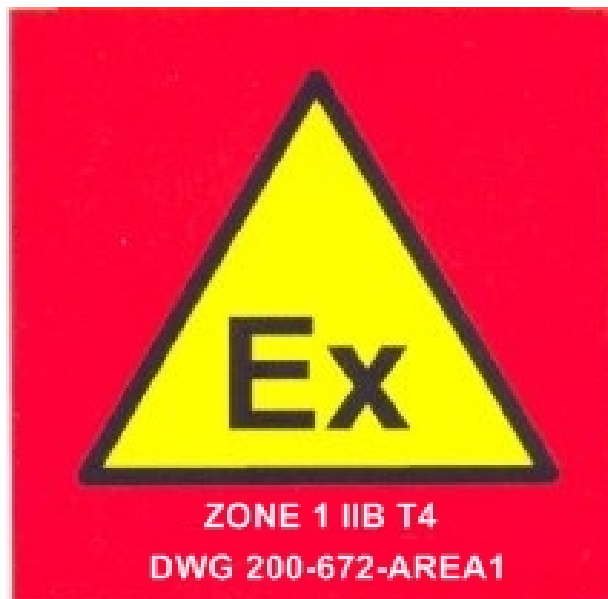
Fig. 14 An alert sign for hazardous locations
