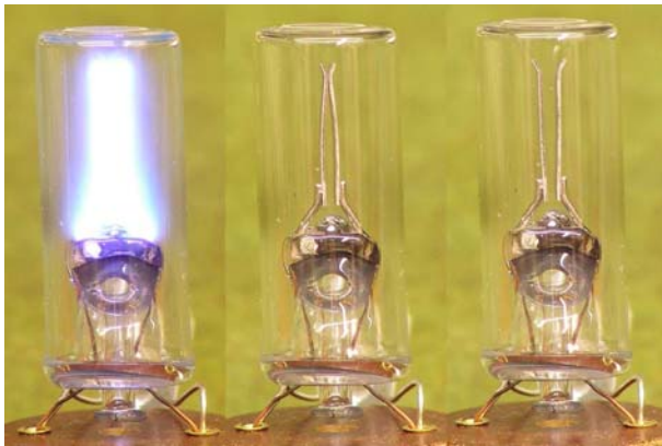
Fig. 3.8: Glow discharge heats up bimetallic contacts, contacts short out glow discharge, cool down again and open ...
