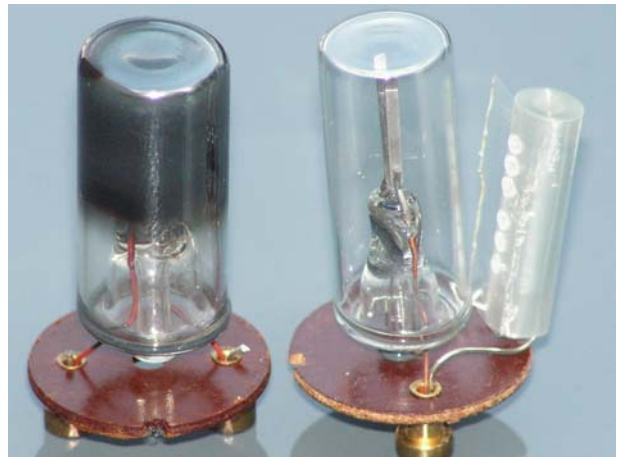
Fig. 3.9: ...and when this game has been going on for long enough, this can be clearly seen when opening the starter (left; on the right an unused sample with filtering capacitor)
