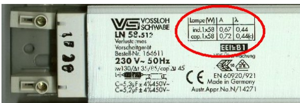
Fig. 5.2: The power factor is always indicated on a ballast
