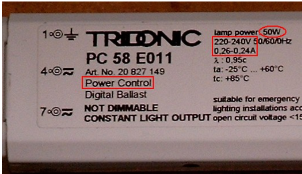
Fig. 7.6: An advantage of electronic ballasts: Offset of voltage variances. Potential disadvantage of this: Current intake increases as voltage sags
