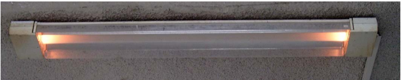
Fig. 3.10: In the end of a day (or a week or a month) the contacts weld together, and the lamp persists in permanent pre-heating operation
