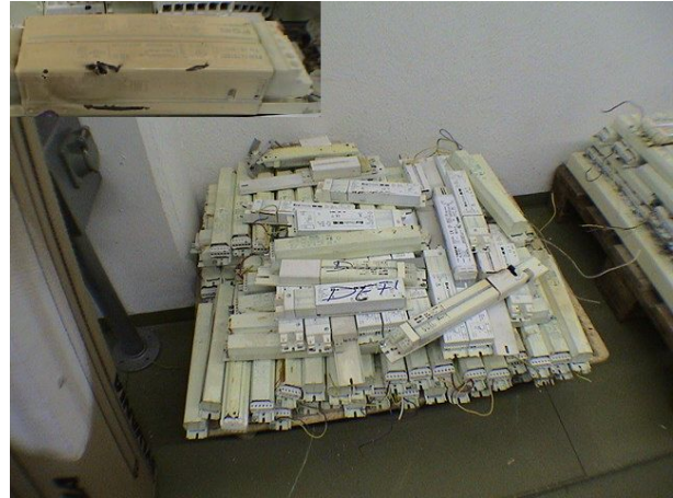
Fig. 7.7: Electronic ballast failures at Swiss Federal Institute of Technology Zurich within one year
