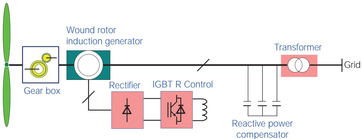
Figure 3-7 | Topology of a variable-slip induction generator (SGCC)
