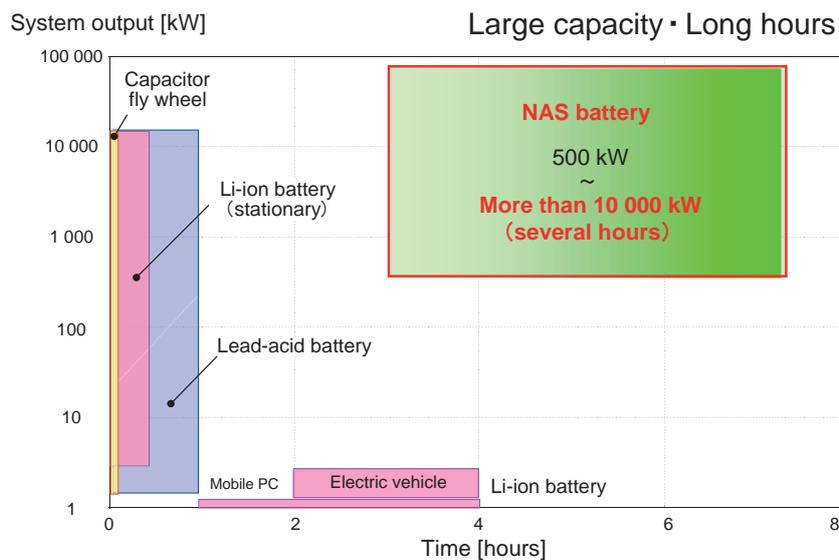
Figure 5-6 | Comparison of battery output and duration (NGK)
