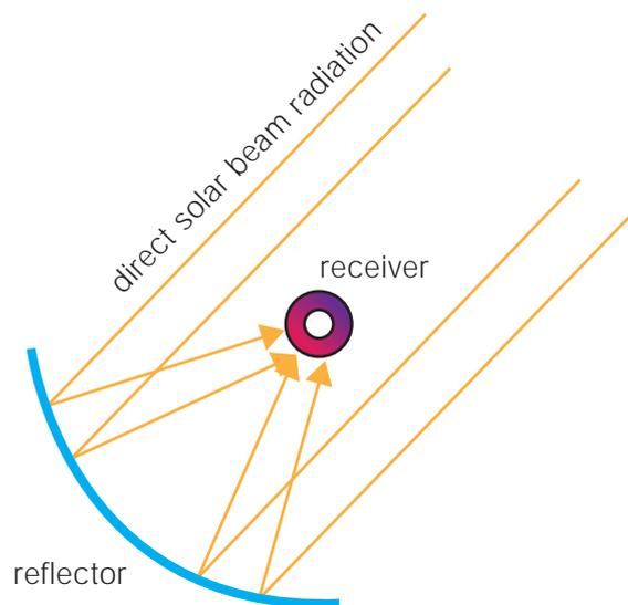
**Figure 3-14 | Principle of obtaining thermal energy in CSP [dlr05]**
