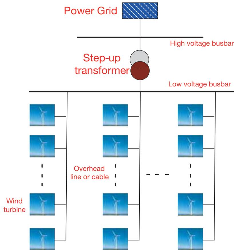
Figure 3-5 | Structure diagram of a wind farm (SGCC)
