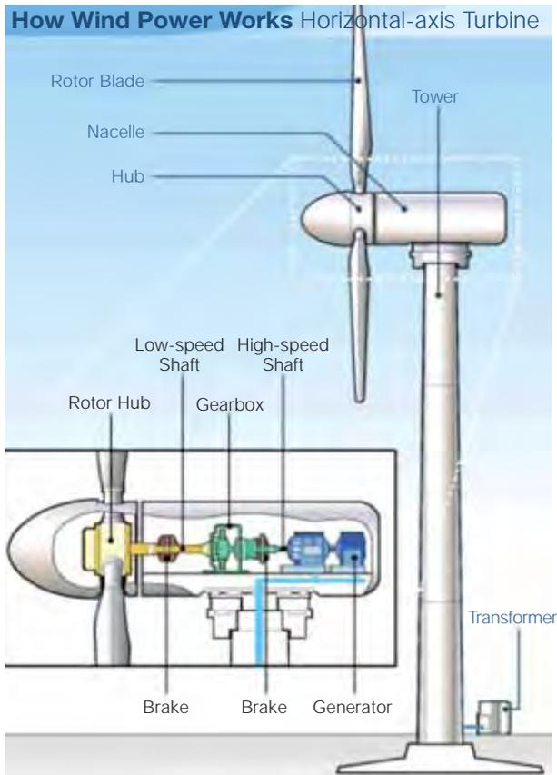
**Figure 3-2 | Structure diagram of a WTG**
