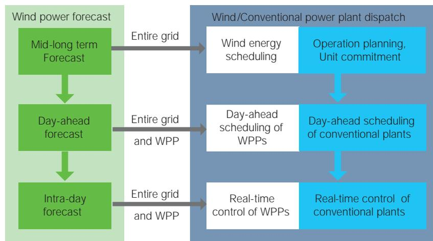
Figure 3-22 | System operation in China taking wind power into account [sgc11]
