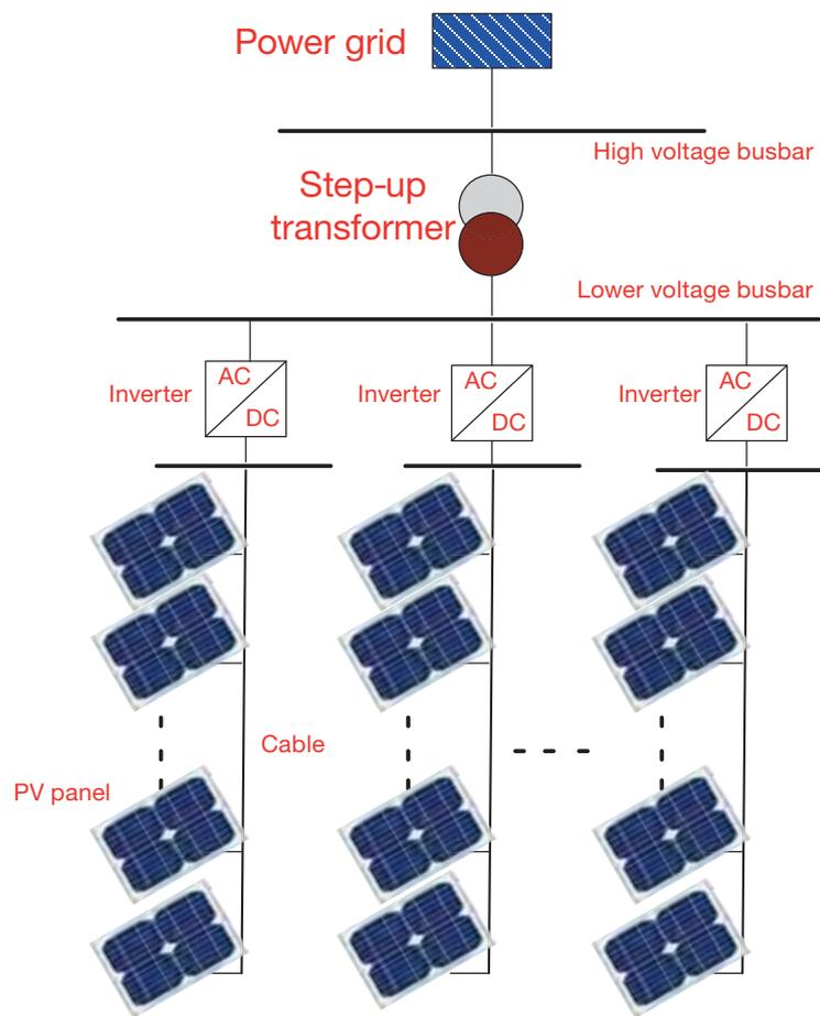
Figure 3-11 | Structure diagram of a PV power station
