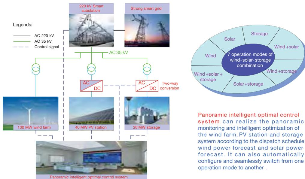
**Figure 5-2 | Architecture of the national wind power, solar power, energy storage and transmission demonstration project, Phase I (SGCC)**
