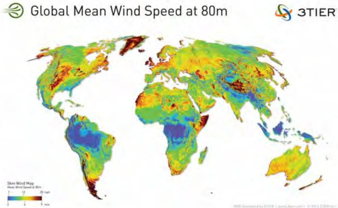
Figure 2-19 | Global mean wind speed at 80 m altitude [tie12]
