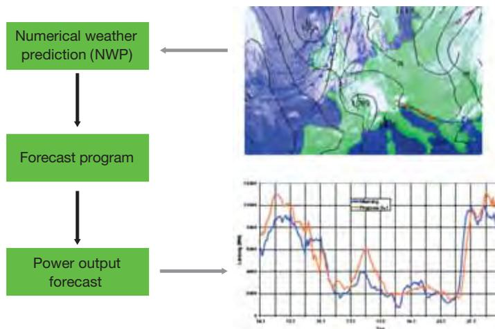
Figure 3-19 | Principle of short-term wind power forecasting (SGCC)
