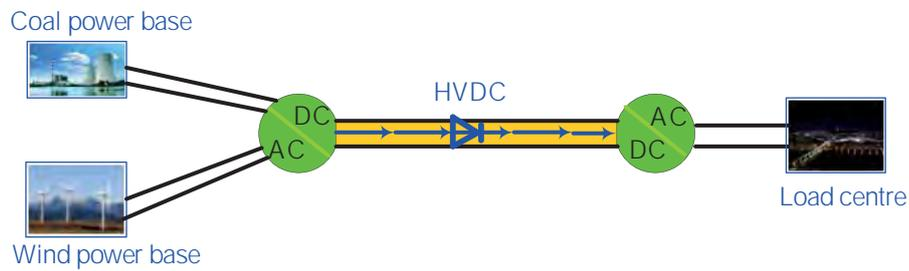
**Figure 4-9 | “Wind-fire bundling” design with HVDC transmission (SGCC)**
