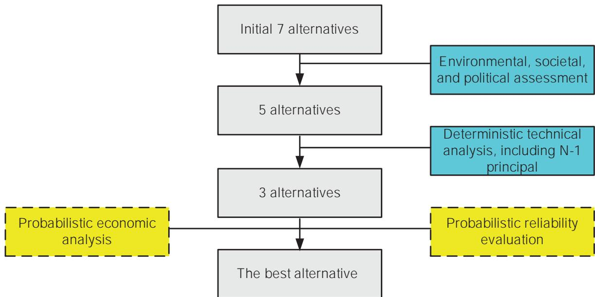
**Figure 4-13 | Conceptual flow chart of probabilistic transmission planning [pts11]**
