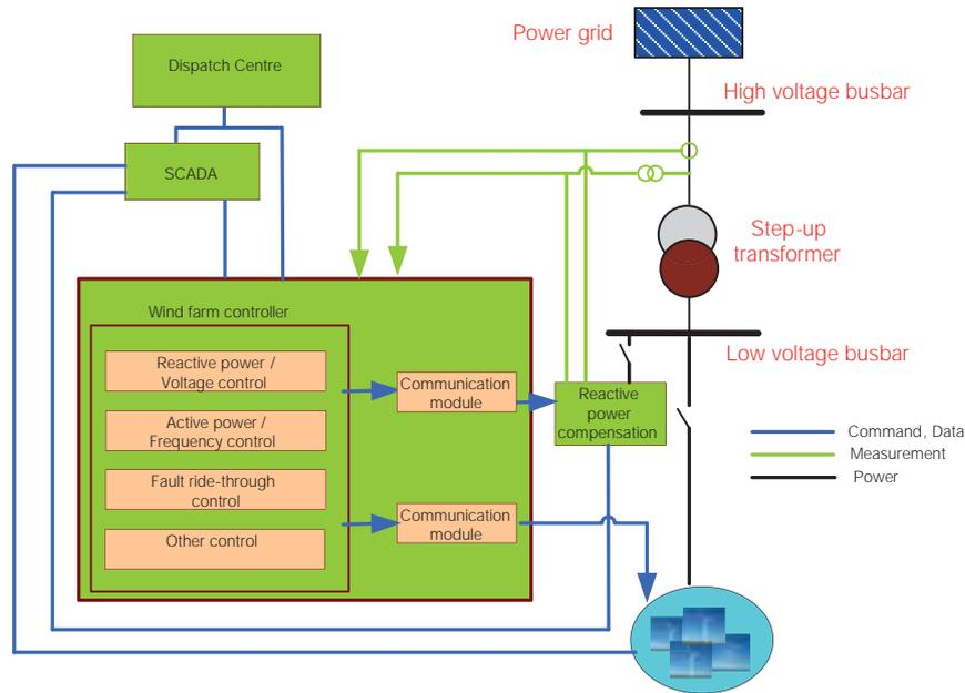
**Figure 4-2 | Typical structure of a “grid-friendly” wind power plant (SGCC)**
