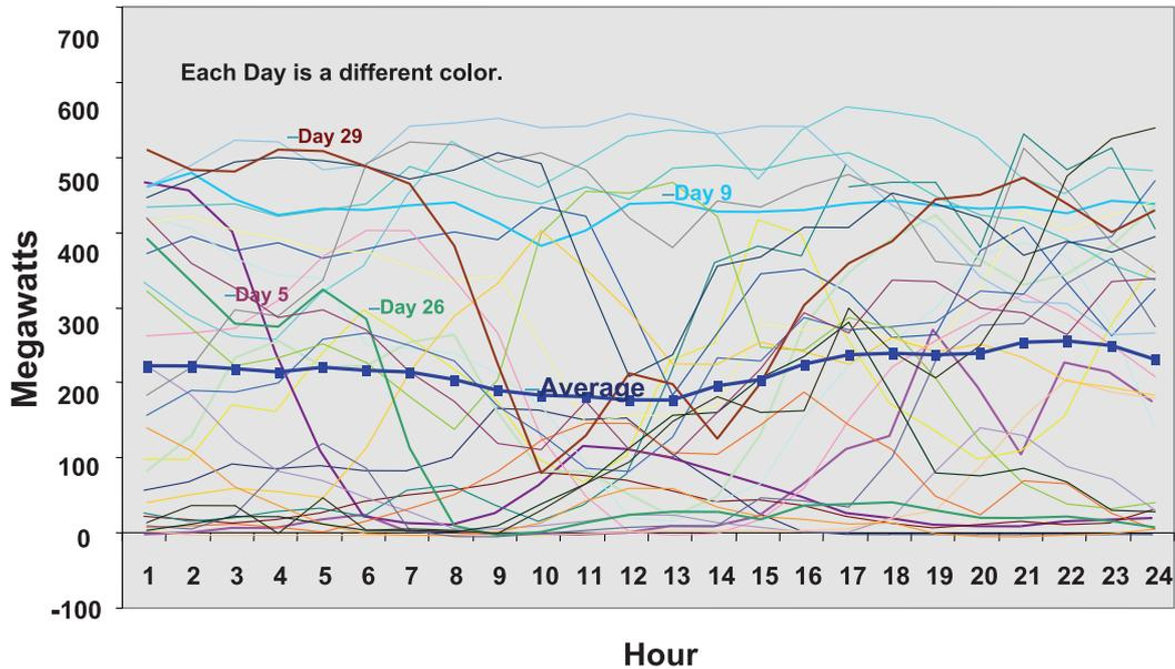
**Figure 2-17 | Hourly wind power output on 29 different days in April 2005 at the Tehachapi wind plant in California [haw06]**
