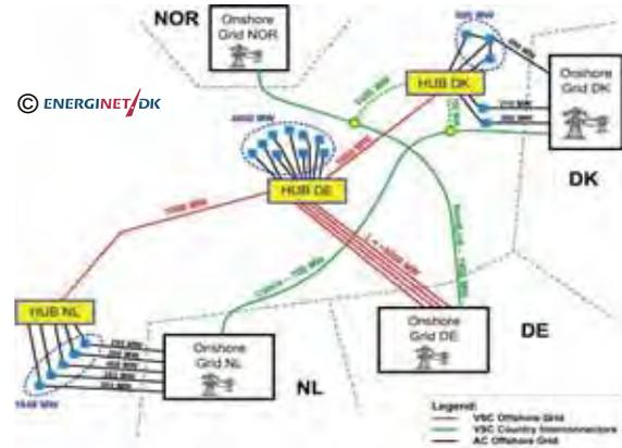
**Figure 4-12 | Benchmark test system for the European transnational offshore grid [coc11]**
