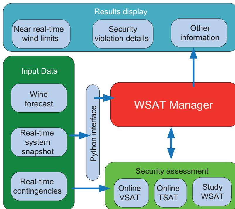
**Figure 4-15 | Wind Security Assessment Tool (WSAT) structure [sin12]**
