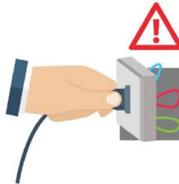
Figure 6 – Loose contacts, e.g. with a loose socket that was kept on being used, can increase the resistivity, leading to a hot spot and a potential source of fire.
