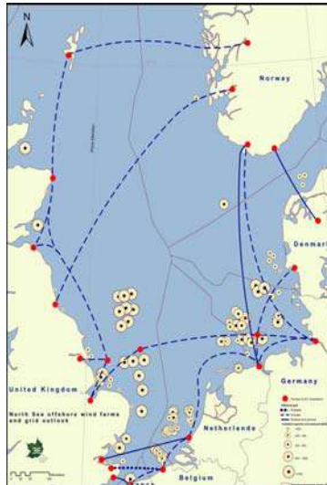
Figure 1 Impression of transnational off-shore HVDC grid interconnecting various EU countries
