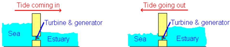
Figure 8 Tidal energy conversion concept
