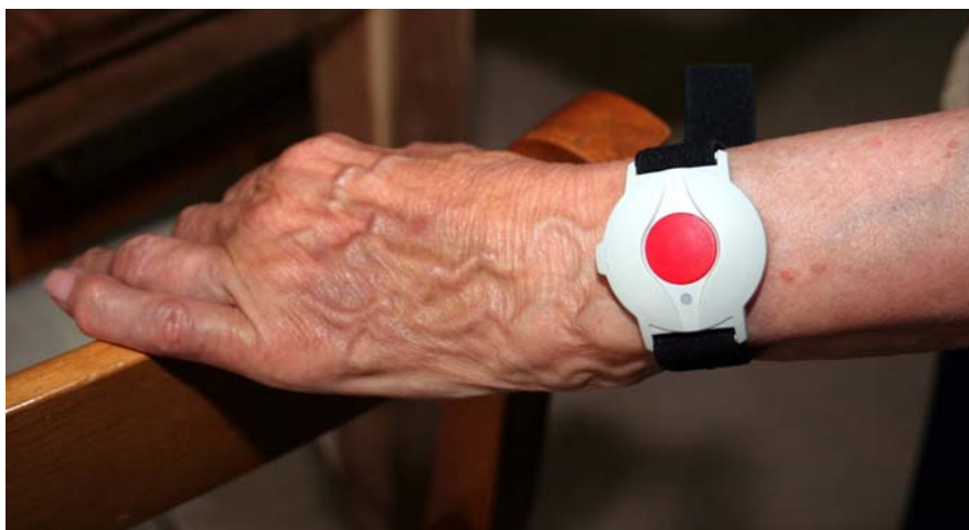
Figure 6: Using the wristband transponder, the resident can activate an alarm when he (she) feels unwell. (Illustration source: E&D Systems)
